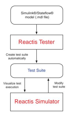
Reactis is an embedded software design automation tool suite – a collection of applications supporting the efficient production of high-quality control software. Reactis currently consists of two components:
